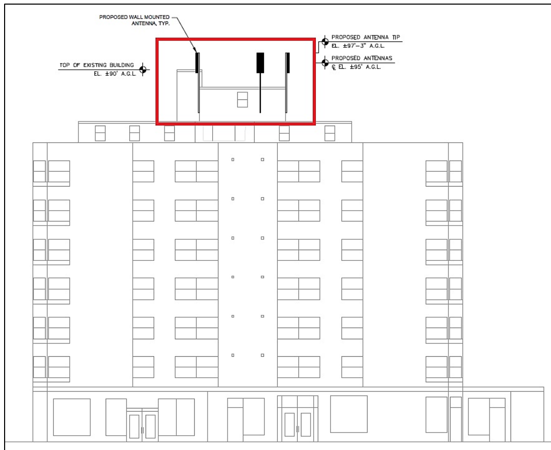
Figure 1: Construction schematic of proposed antenna installation
